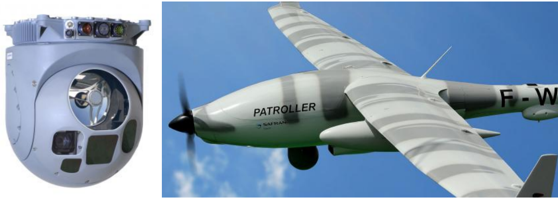
Figure 5: Euroflir 410 (left), last generation of ultra-long-range electro-optical system commercialized by Safran. Its navigation system includes the first commercial implementation of an Invariant EKF. It is embedded in particular in the drone Patroller (right).
