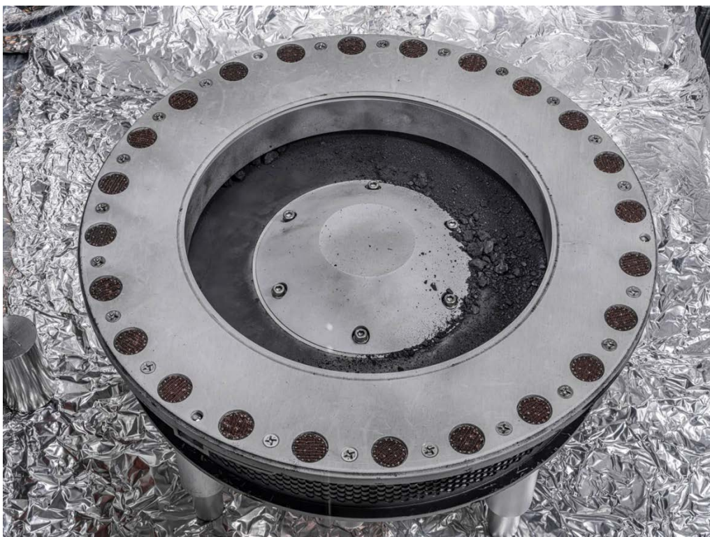
Fig. 13. Sample container of OSIRIS-Rex Touch-and-Go Sample Acquisition Mechanism. Contact pads around ring (between screws) are \sim 17 mm in diameter. In the inner ring, small pebbles can be seen at upper left holding open the mylar flap. Pebbles and fine particulates are visible on top of the mylar flap at right. The presence of coarse and fine particles confirms remote sensing interpretations. Image source: https://www.asteroidmission.org/?latest-news=nasas-osiris-rex-achieves-sample-mass-milestone
