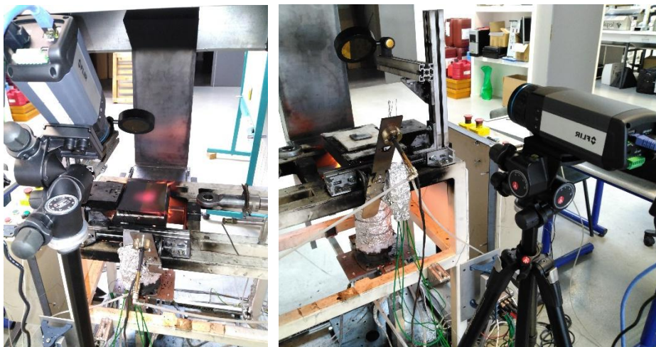
Figure 1. Experimental fire bench: direct oblique view on steel plate (left) and normal reflected view on a composite laminates (right) subjected to a kerosene flame
