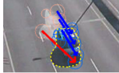
Fig. 6. Each arrow is obtained by feature tracking through SURF and FLANN algorithms. The red arrow indicates a match between features that has been filtered out by the angle filter.
