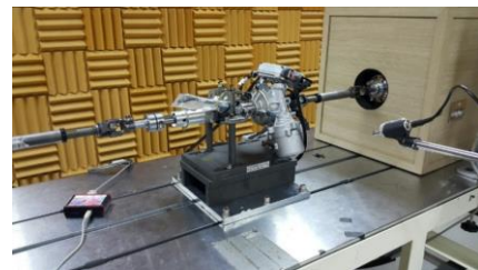
Figure 3. Evaluation setup for operational noise
