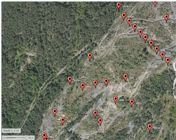
Figure 6. Reflectors on the central part and location of the stable crest at the La Valette landslide (France)
