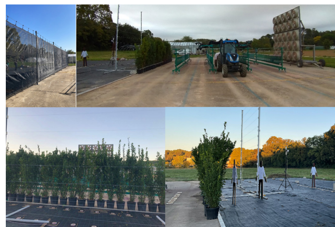
PHOTO 1. EoleDrift test rig and the physical barriers tested: FilPack “bv 106” artificial net, top left; and bay hedge, top right and bottom.
