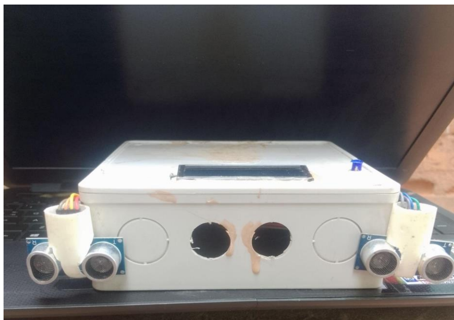
Fig. 10. Ultrasonic Sensors Positioned at Entry and Exit
