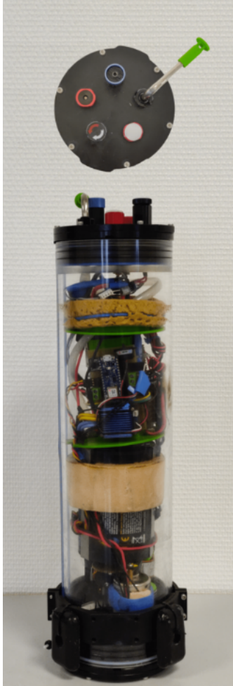
Figure 1: The float system. On the top cap, clockwise: Pressure valve, Water inlet, LED, ON/Off button, Bar02 Pressure sensor
