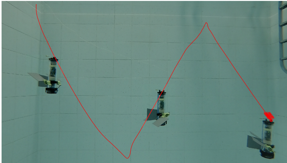
Figure 2: The float equipped with passive mobile wings on a slope-trajectory tracking mission. Three photos of the float are superimposed to show its forward movement. The red line represents the trajectory of the float in the (x_0, z_0) plane
