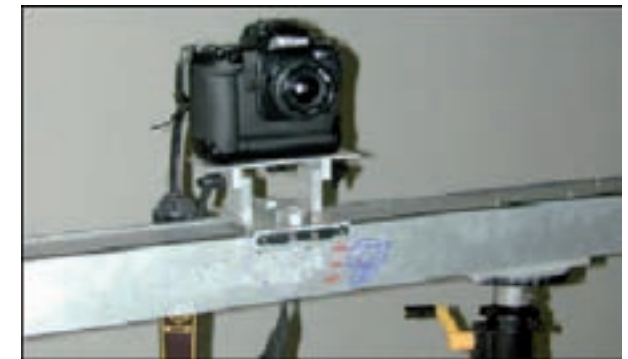
Fig. 2. Calibrated aluminium bar on which the digital photcamera used for the photogrammetric survey was positioned.. [ www.menci.com ]
