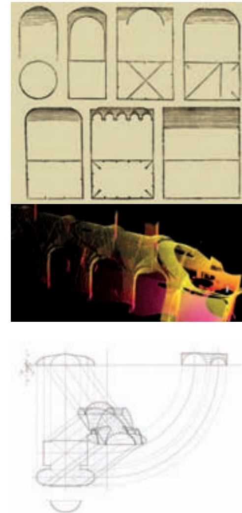
Fig. 9. Some examples of vaults : (a) – palladian vaults, (b) – points’ cloud of the cross vault of the Tolentini (c) – geometric analysis of the cross vault of the tablinum in the Convento della Carità , [A. Palladio, “I Quattro Libri dell’Architettura”, Domenico De’ Franceschi, Venezia 1570, I, p. 54; aut. A. Sdegno and P. Vernier, 2006; aut. A. Sdegno, 2003]
