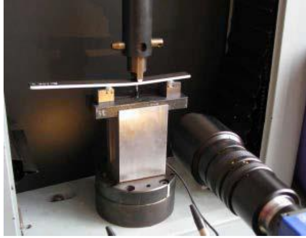
Figure 19. Application of the standard ASTM D7905 for the ENF test for laminated composites [44],[79].
