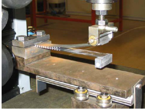
Figure 23. Application of the standard ASTM D6671 using the MMB test for laminated composites [44],[90].
