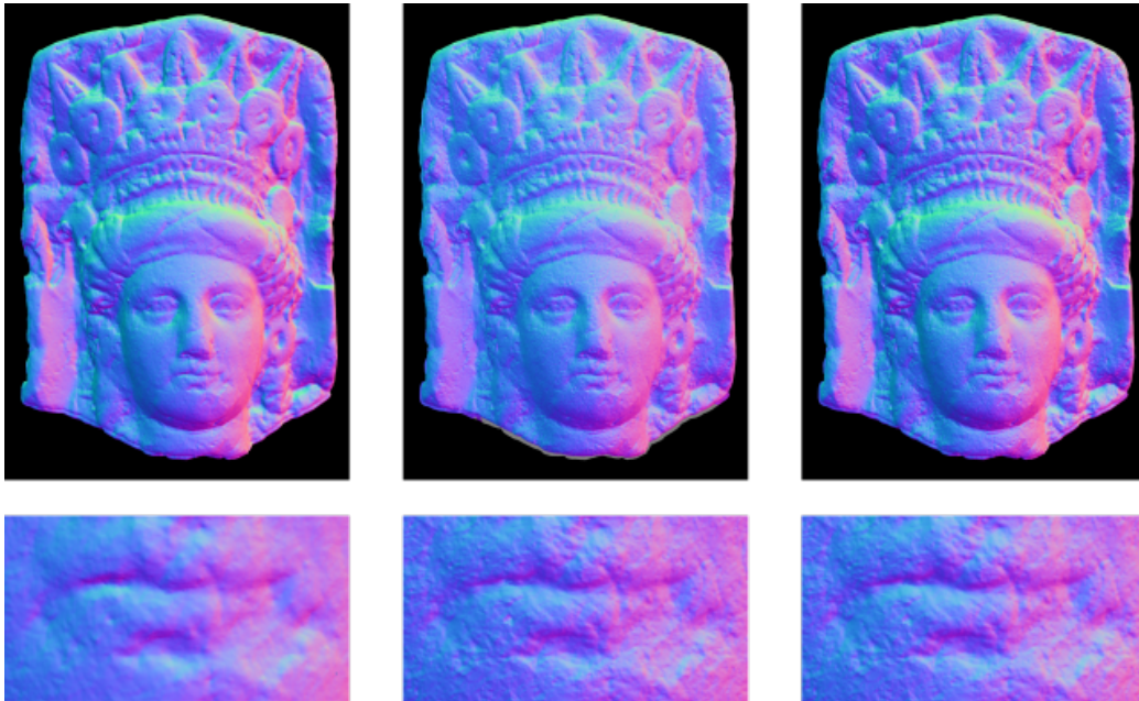
Figure 7: Three 3D reconstructions of the Cypriot head, shown as normal fields in RGB representation: Photogrammetry using Metashape software (left); Calibrated PS using an RTI dome (center); PG+PS (right). The bottom line shows zooms of the mouth area.
