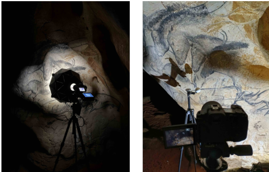
Figure 4: Implementing the digitization of the Panneau des Chevaux using calibrated photometric stereo. Left: Use of an RTI dome, for which the lighting has been pre-calibrated. Right: Use of a white sphere to calibrate lighting a posteriori.
