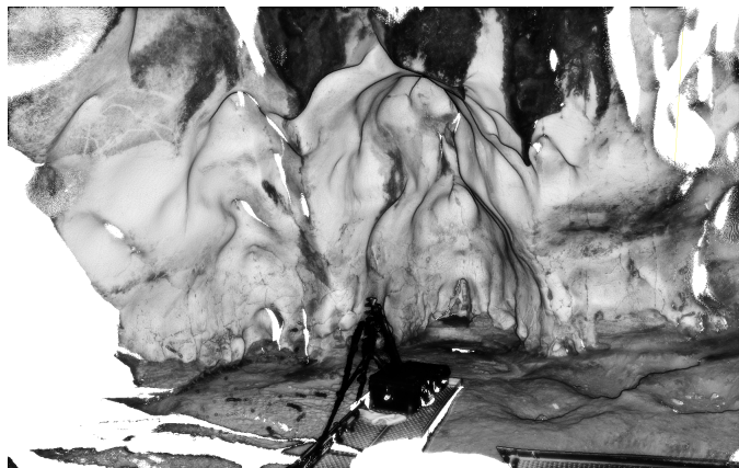
Figure 3: 3D point cloud of the Panneau des Chevaux obtained with a TLS scanner. The grey levels of the signal intensity are weakly representative of the RGB color of the wall. Credit: Perazio Engineering, French Ministry of Culture.
