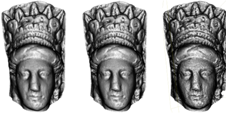
Figure 8: Three 3D reconstructions of the Cypriot head, represented as triangular meshes: Hand-held scanning (left); Photogrammetry using Metashape software (center); Multi-view PS (right), which is the method described on the diagram in Figure 9.
