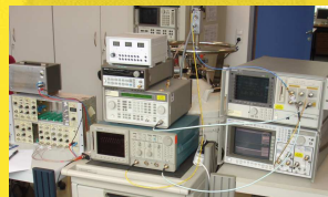
Figure 10: System set-up including: Sine-wave clock generator with dc-block, sampling oscilloscope and two dc-power supplies of RSFQ and amplifier part.
