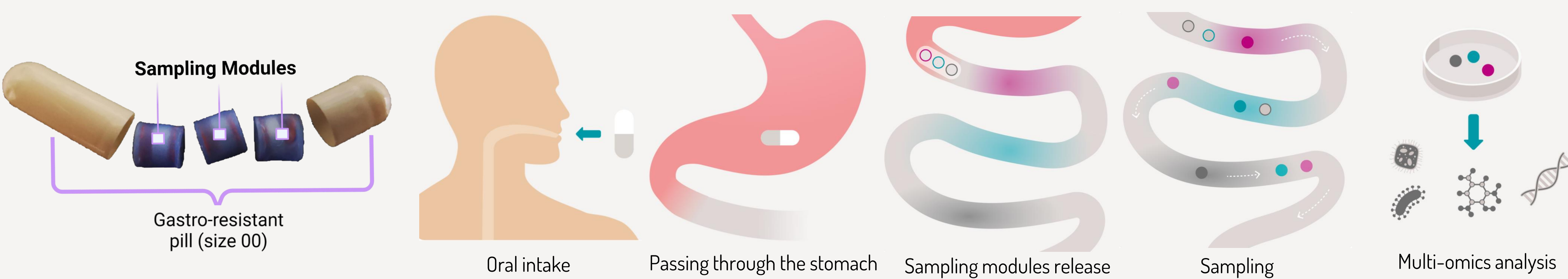
Figure 1: Structure and use of Pelican Sampler medical device (MD)
