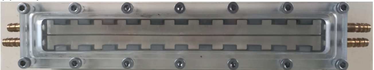
Figure 11: Fabricated (a): TO-optimized, (b): Benchmark and (c): Simplified HX units using the water jet cutting process.
