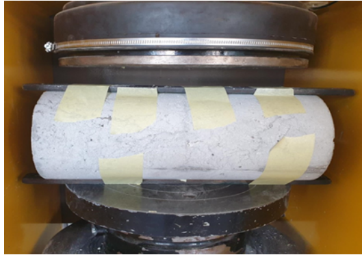
Fig. 11. A SFRC sample during the Brazilian destructive test.
