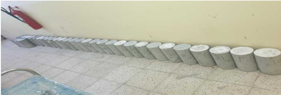
Fig. 10. Set of samples with random fiber distribution.
