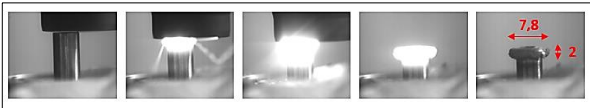
Figure 12 - Friction forming of the rivet head at 12000 rpm and 6 mm/min
