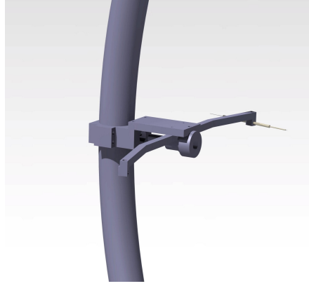
Fig. 3 CAD image of the Langmuir probe setup. The LP is not aligned with the rotating arm.
