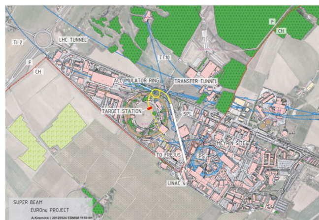
FIG. 2. Layout of the Super Beam facility at CERN. The yellow line shows the transfer lines from SPL and the accumulator ring, while the red box shows the location of the target station, in the ISR area. (Image provided courtesy of Elena Wildner and the CERN Civil Engineering Service.)
