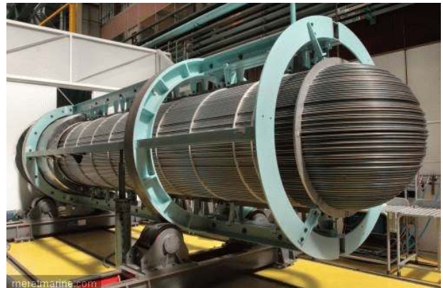
Figure 1 – Tube heat exchanger (meretmarine.com)
