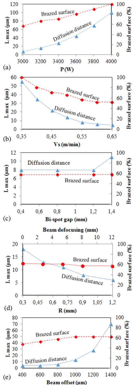
**Figure 8.** Evolution of diffusion distances and brazed surface % in function of heat source parameters: laser power (a), linear laser speed (b), gap between the spots (c), beam defocusing (d) and beam offset from joint line to Ti side (e).
