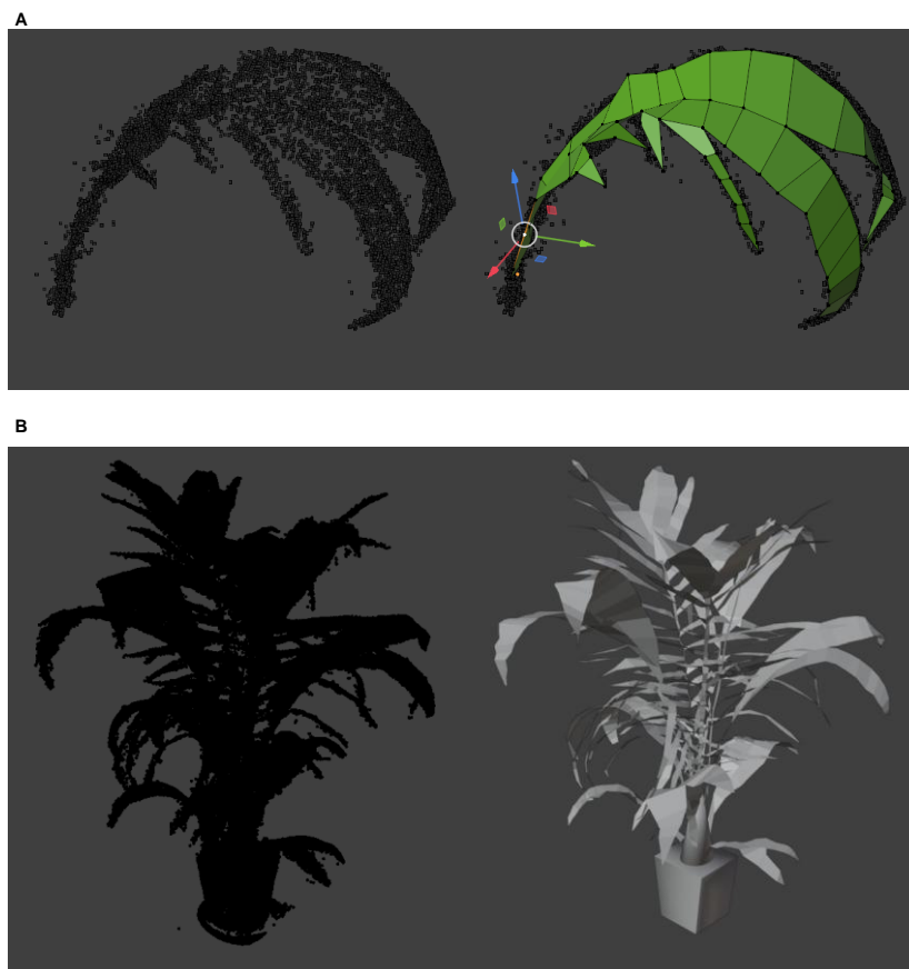
262 263 Figure 6: 3D reconstruction from LiDAR point clouds. A) Building plane meshes on point cloud with the poly build 264 tool of Blender. B) Full reconstruction of the 3D mock-up from points cloud.
