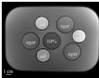
Fig. 2. Magnitude image depicting the experiment: the emulsion tube is surrounded by 3 agar tubes to correct for B_0 drift and 3 vials of pure peanut-oil.
