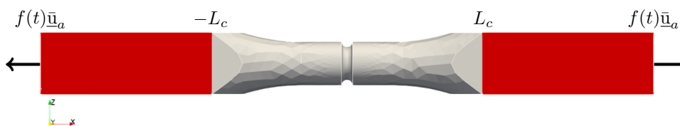
(a) Notched structure, with displacement \bar{u}_a at f = 1 scaled by f(t) on highlighted red regions, in opposite directions
