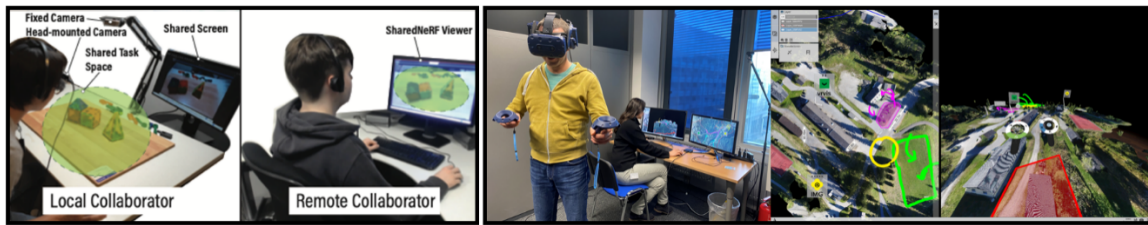
Figure 9: Illustrations of the dimensionality asymmetry: on the left, the local collaborator manipulates a set of 3D physical objects, while the remote collaborator performs 2D interaction on a video showing the remote set of objects [72]. On the right, VR is used to provide one of the collaborators with 3D visualizations in a tactical resource planning scenario [54], images used with the permission of VRVis GmbH and IMG - Österreichisches Bundesheer.
