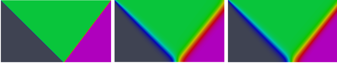
Figure 10.2 – Shock reflection, mesh 140 \times 80 . Exact solution (left), Lattice Boltzmann scheme D2Q5Q4Q4 (middle) and Godunov scheme (right).
