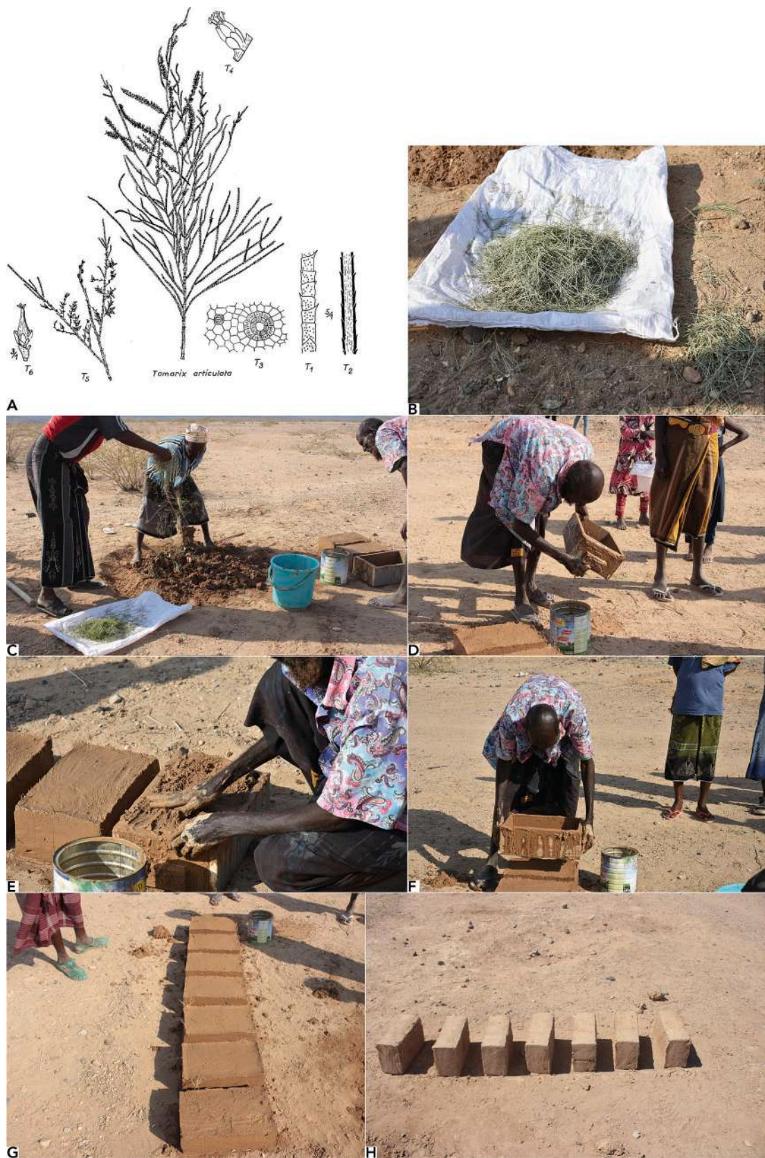
Fig. 2. Sequence of the chaîne opératoire for the molded mud bricks. The temper commonly used is tamarix nilotica (A-B), added to earth and water and mixed with a pick axe (C). The mason wets the internal walls of a bottomless mold (D) before throwing a ball of mud packed down with a fist, the excess earth scraped away by hand (E) before removed from the mold (F). The mud bricks are left to dry in the sun (G), one side at a time (H) during 5 days – Copyrights: Q. Aubourg, E. Baudouin.
