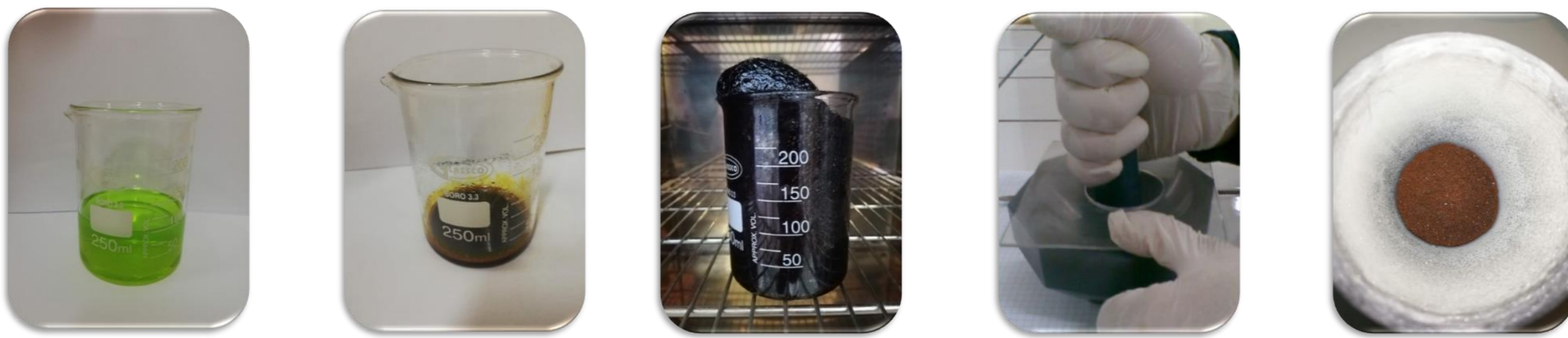
Figure 1 : Steps for preparing powder with sol gel method
