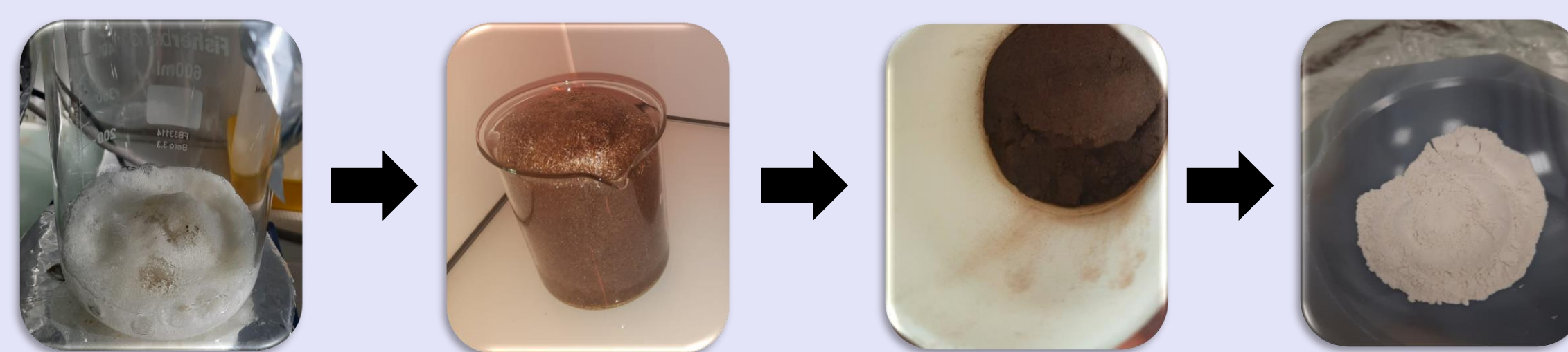
Step 1: Preparing the powder with sol gel synthesis method
