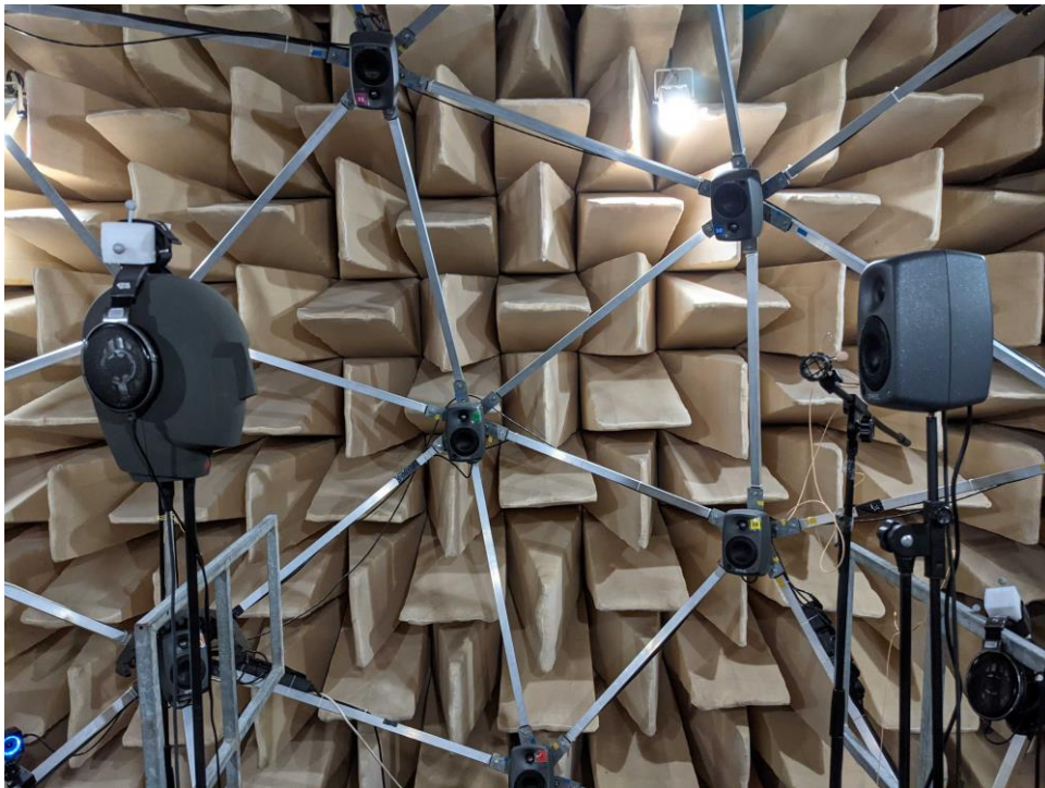
Figure 10. Acoustic source (loudspeaker with head-worn microphone 5 cm apart) and receiver (artificial head wearing headphones) located 1 m apart in the experimental room, used for the adjustment of the auralisation system playback level. Source: photograph by the authors.
