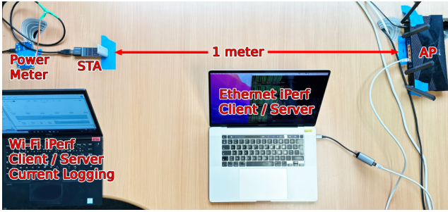
Fig. 1: 802.11ac/ax Current Measurement setup
