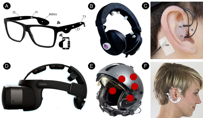
Figure 12. Examples of unobtrusive EEG sensing systems for BCI applications. A: Dry EEG sensors embedded in glasses frames (adapted from Sopic et al., 2018). B: Headphones-mounted wet-sponge EEG electrodes (Smartfones from mBrainTrain, Serbia). C: In-ear electrodes (adapted from Bleichner et al., 2015). D: Dry EEG extension of a Virtual Reality headset (Galea from OpenBCI, New York). E: Prototype of a flight helmet fitted with EEG sensors (red dots represent possible electrode locations inside the helmet). F: Around-the-ear EEG array (adapted from Bleichner and Debener, 2017).
