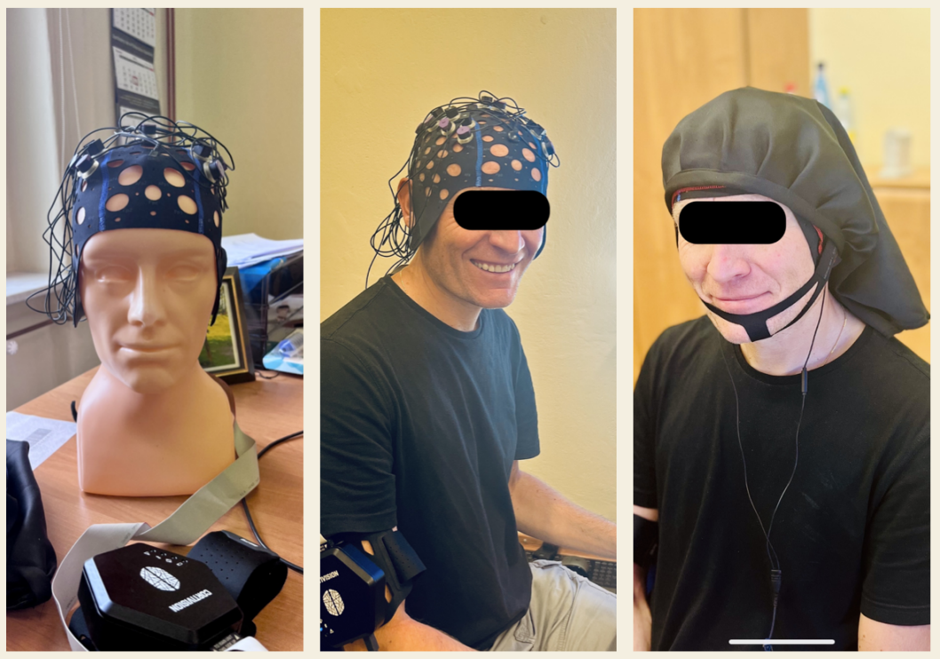
Fig. 4. A representative fNIRS headset from Cortivision (left and middle) with appropriate cover for proper recordings (right).
