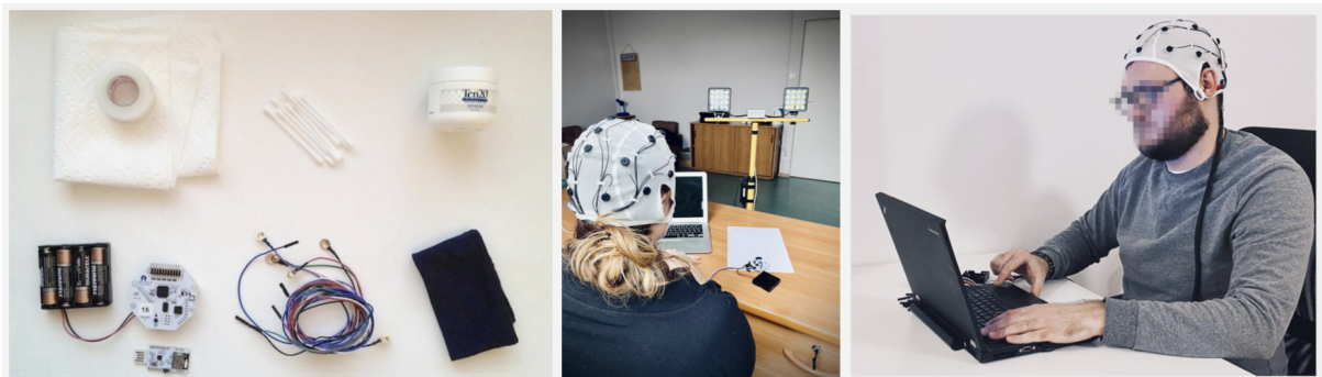
Fig. 3. A representative low cost EEG headset from OpenBCI, New York.
