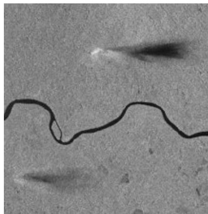
Figure 3. Effect of a rainstorm on a SIR-C radar image in X band over Pará state, Brazil. Source: NASA.
