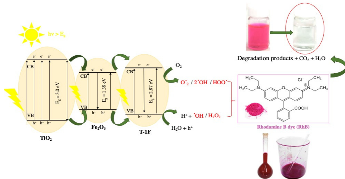
Figure 14. The suggested mechanism of RhB degradation using TS-1F under sunlight.
