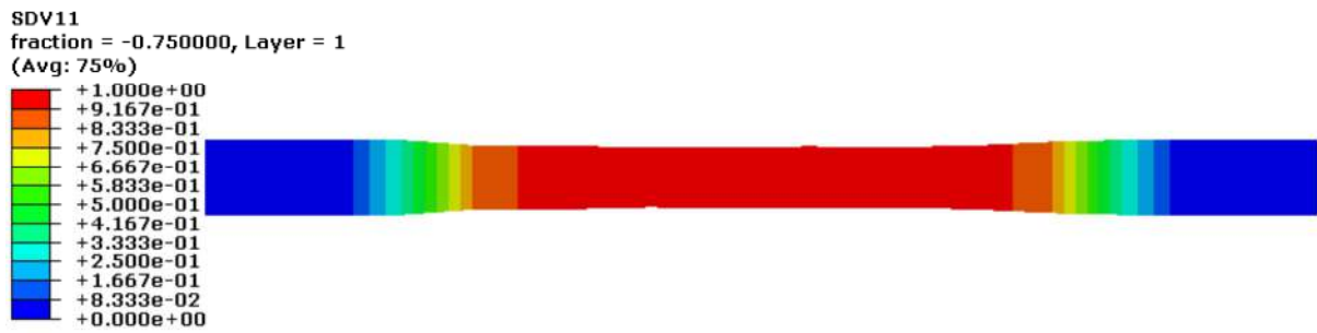
Figure 3. Localization of damage ( d_{12} ) in test specimen – shear test.
