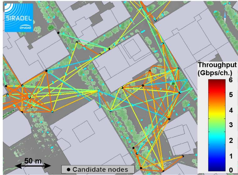
**Figure 2.** Mesh links in the outdoor backhaul network.
