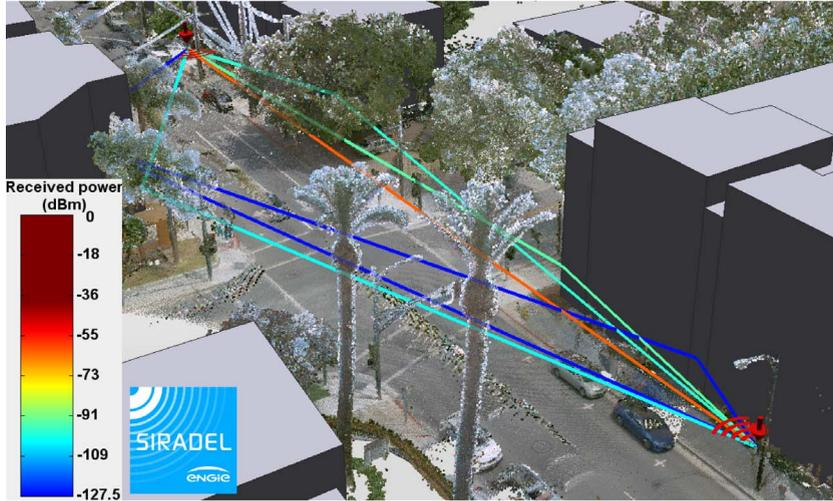
**Figure 1.** Multi-path propagation considering fine 3D tree's representation.
