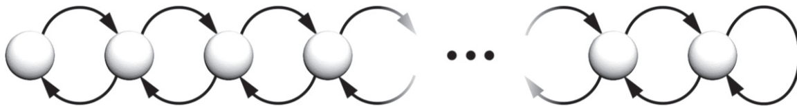
Figure 7. Sketch of the cellular automata for the U(1) QLM with N rishons on the link, where N + 1 is the number of nodes in the picture. The rightmost node, the only one with a self-pointing arrow, is the one related to charge q = \lfloor N/2 \rfloor .
