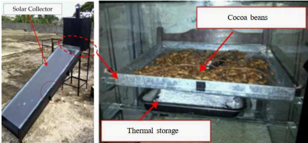
447 Figure 12: Sorption bed located inside the drying chamber - Application of adsorbent (zeolite X) as thermal storage in a natural 448 convection indirect dryer for cocoa beans drying [89]. Adapted from Case Studies in Thermal Engineering 5 (2015), Sari 449 Farah Dina, Himsar Ambarita, Farel H. Napitupulu, Hideki Kawai, Study on effectiveness of continuous solar dryer integrated 450 with desiccant thermal storage for drying cocoa beans, Pages 32–40, Copyright (2014), with permission from Elsevier.
