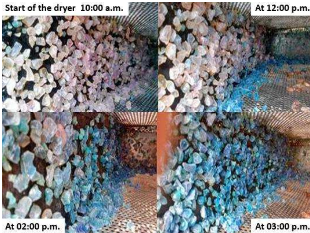
308 Figure 5: Indicating silica gel bed used as thermal storage in a forced convection solar dryer in India [90].
