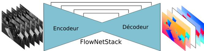
FIGURE 2 – Architecture *FlowNetStack*.
