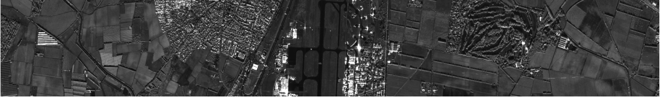
Figure 3 SETHI SLC SAR Image. HH polarization. X-band. Range direction is on the vertical axis and the azimuth direction is on the horizontal axis.
