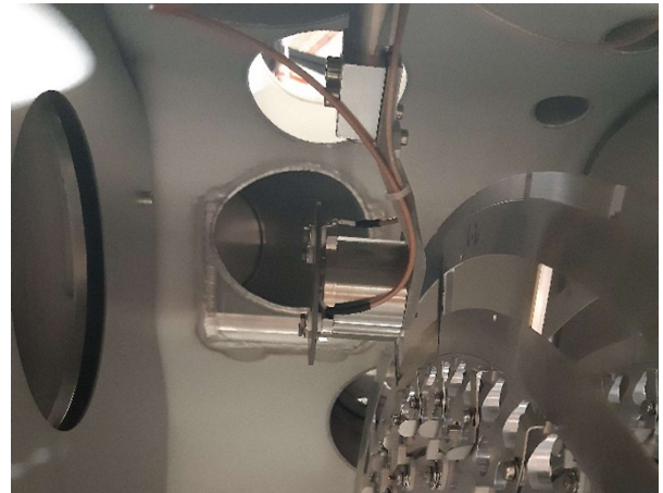
Fig. 3. View of the Faraday Cup for the HI beam.
