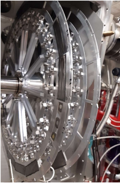
Fig. 1. View inside the chamber of the two wheels with their respective six sectors and targets or charge equilibration carbon foils mounted.
