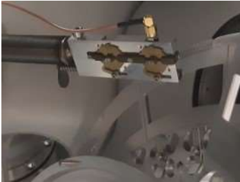
Fig. 5. View of the upper part of S 4 TS with the scattered particles detectors, sectors of the first wheel are removed
