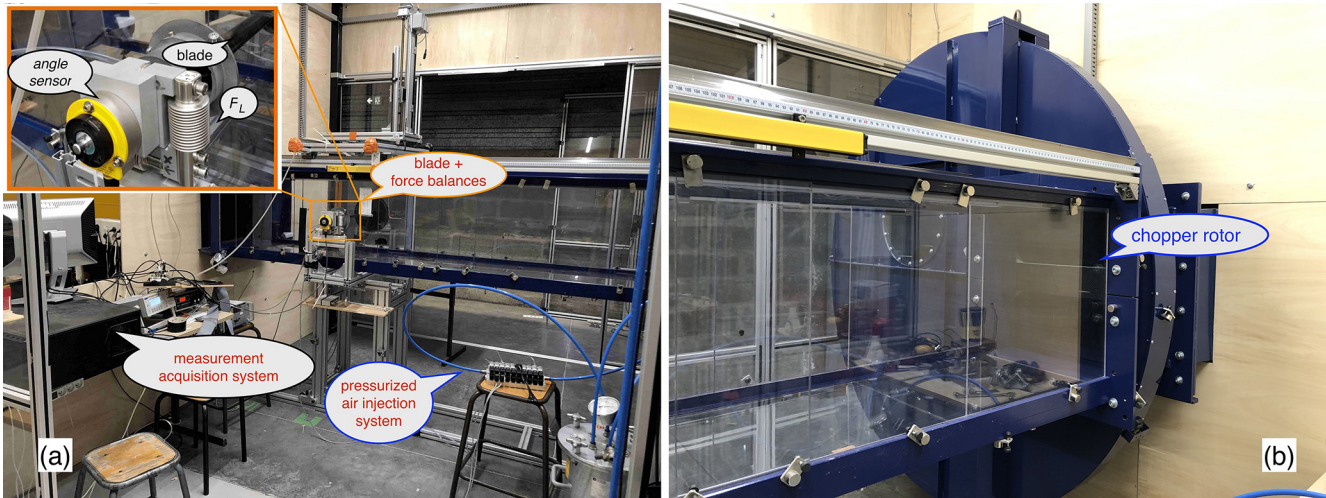
Figure 1. The wind tunnel test bench is composed of the following: (a) the test section with all needed instrumentation (blade, load measurement system, angle sensor, acquisition and actuation systems) and (b) the perturbation system, also called the chopper (see Neunaber and Braud, 2020). The actuation system consists of a pressurized air circuit (blue tube) that is connected to a first reservoir on the bottom right of the image and to the solenoid valves set on the stool. Two vinyl tubes are connected from the exit of two solenoid valves to the ends of the hollow tube inside the blade. Reproduced from Michel et al. (2024).
