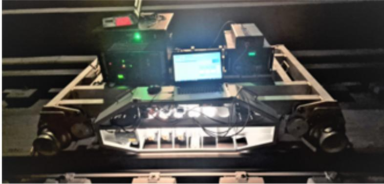
Fig. 1: EMAT trolley for online rail inspection.
