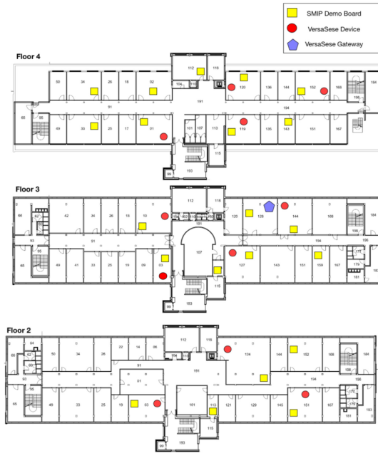
Fig. 9. Default topology of the physical testbed, spanning throughout three building floors.
