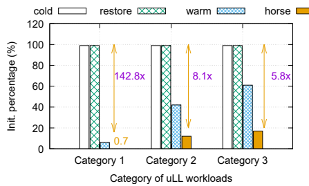
Figure 4: Sandox initialization percentage in the trigger process of 3 uLL workloads for four scenarios. HORSE outclasses warm by up to 8,95 \times , restore by up to 142,7 \times , and cold by up to 142,84 \times .
