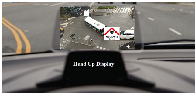
Fig. 6. Head up Display receiving the edge processed information in the hazard location
