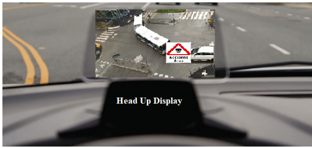
Fig. 12. Head up Display receiving the edge processed information in the hazard location
