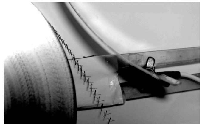
Fig. 7. High-speed camera recordings of the trajectory of copper particles for U = -17 kV, d_1 = 7 cm, d_2 = 4 cm, \alpha_1 = 10^\circ , \alpha_2 = 45^\circ , n = 70 rpm and f = 100 Hz.
