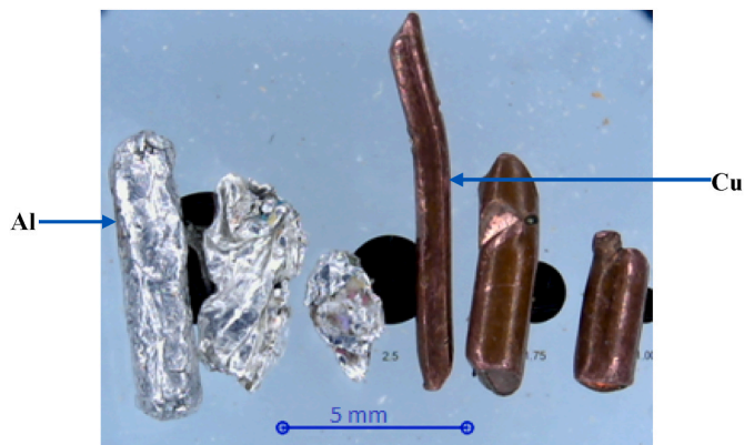
Fig. 1. Cu and Al particles picked up from the WEEE processing at Environmental Recycling Company, France.
