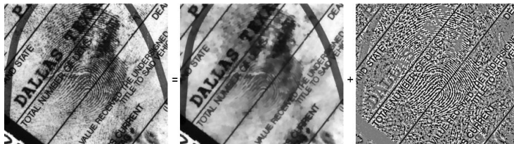
Figure 9: Extraction of a fingerprint from a document with the TV+L^1 model
