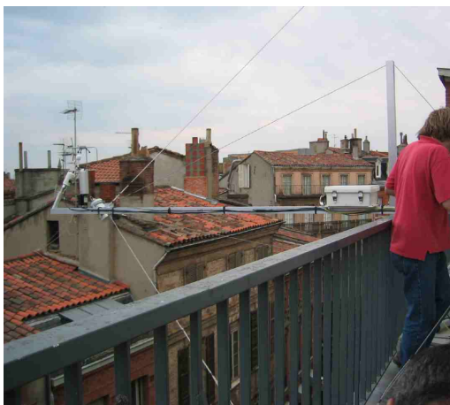
Figure 3: Pictures of the booms employed to measure CO 2 fluxes at rooftop level during the CAPITOUL campaign. Credits : CNRM.
